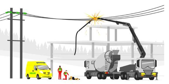
High-voltage lines are extremely dangerous, even when you are many metres away. Touching high-voltage lines and installations has led to many near-misses and tragic fatal accidents.
